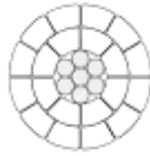
Compact wire KUSIL-AIS with trapezoidal conductor and steel core.
